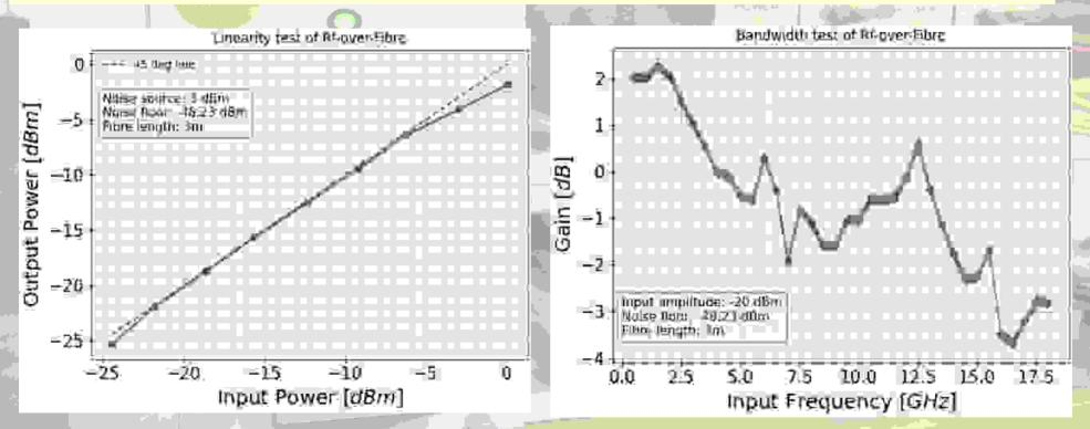
Rf-over-fibre linearity and BW with manual frequency sweeping and network analyzer
