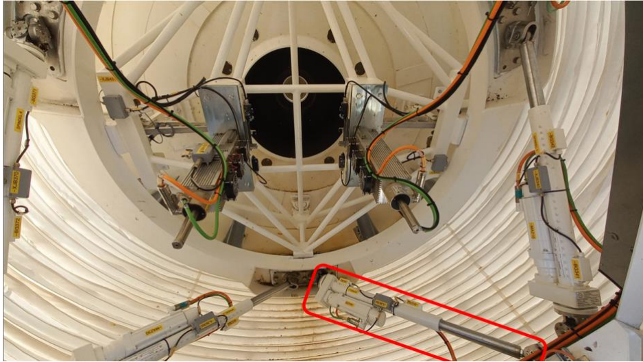
Figure 5: Subreflector hexapod control and detail of the blocked spindle.
