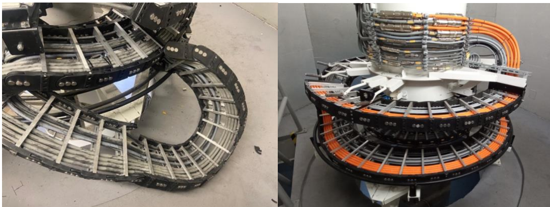
Figure 6: Detail of 13m cable wrap after the failure (left) and after the repair (right).
