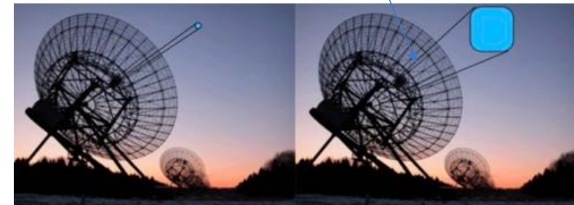
APERTIF Phase Array Feed on WSRT expand FOV by factor of 25
