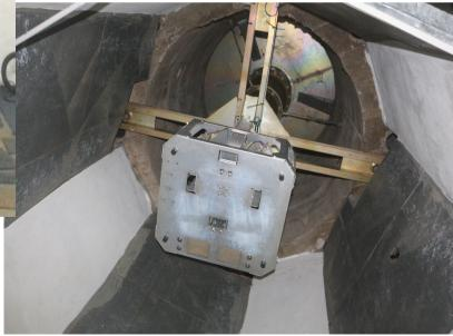
Dual Uncooled receiver (C-band) system at central frequencies of 5 GHz and 6.7 GHz
